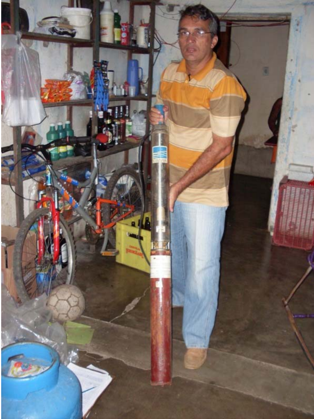
Figure 4.21: Underwater pump from an abandoned alluvium well.
