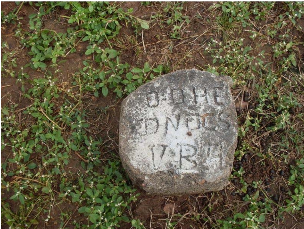
Figure 4.31: Survey marker positioned by VBA on the Lagoa Nova Dam site.
