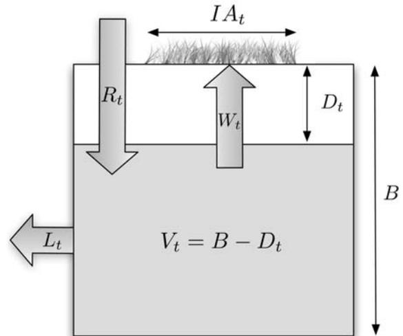
**Figure 6.** Stylized representation of the modeled groundwater budget for a given district (note: district identifier  $d$  is dropped).  $R_t$  is net recharge,  $W_t$  is pumping,  $L_t$  are subsurface losses,  $D_t$  is drawdown, and  $IA_t$  is irrigated area.  $V_t$  is the saturated thickness of an aquifer with mean porosity  $\rho$ . The subscript  $t$  denotes time-dependent variables.
