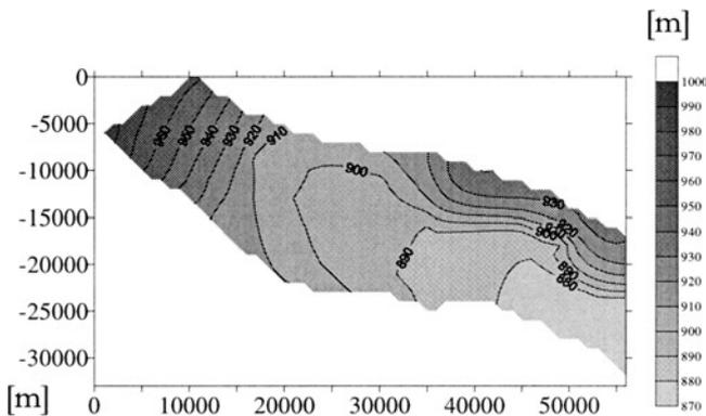
**Figure 7.** First moment of heads in meters (first-order second-moment (FOSM) method, Palla Road Aquifer, conditioned by 10 head measurements).
