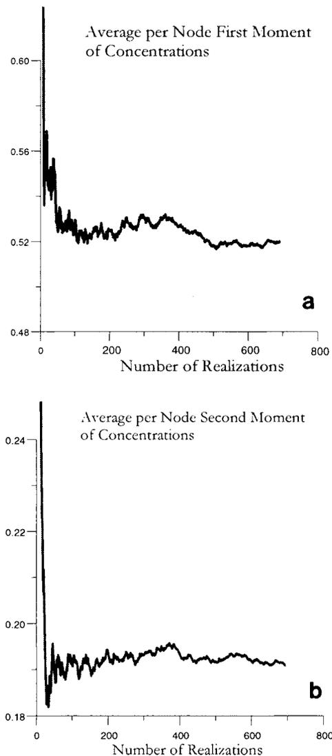
**Figure 13.** Convergence behavior of (a) first and (b) second moment of concentrations (Monte Carlo method, Palla Road Aquifer, conditioned by 10 head measurements).
