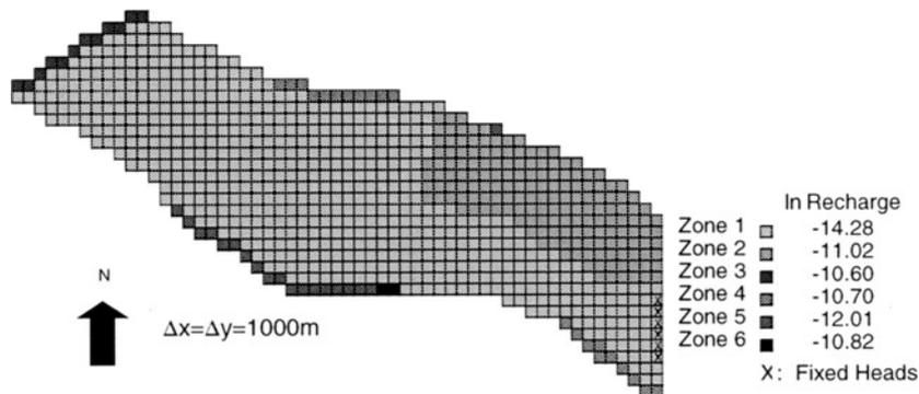
Figure 2. Six recharge and lateral inflow zones of the Palla Road Aquifer with log recharge  $q$  in  $\ln(\text{m d}^{-1})$  were chosen. Fixed-head cells are indicated also.
