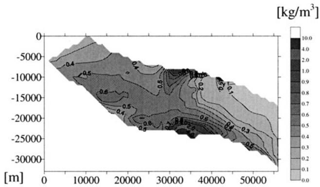
**Figure 10.** First moment of concentrations in  $\text{kg m}^{-3}$  (FOSM method, Palla Road Aquifer, conditioned by 10 head measurements).
