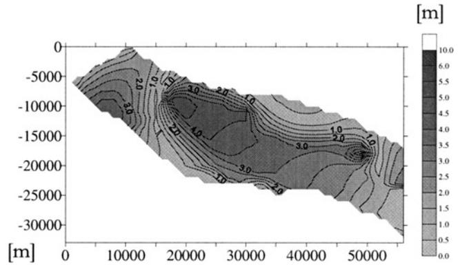
**Figure 8.** Standard deviations of heads in meters (FOSM method, Palla Road Aquifer, conditioned by 10 head measurements).
