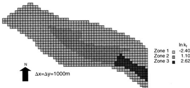
**Figure 4.** The  $\ln k_f$  zones,  $k_f$  given in  $\text{m d}^{-1}$ .
