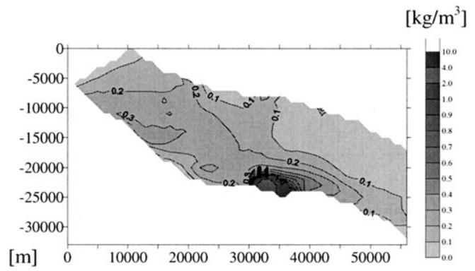
**Figure 12.** Standard deviations of concentrations in  $\text{kg m}^{-3}$  (Monte Carlo method, Palla Road, conditioned by 10 head measurements).
