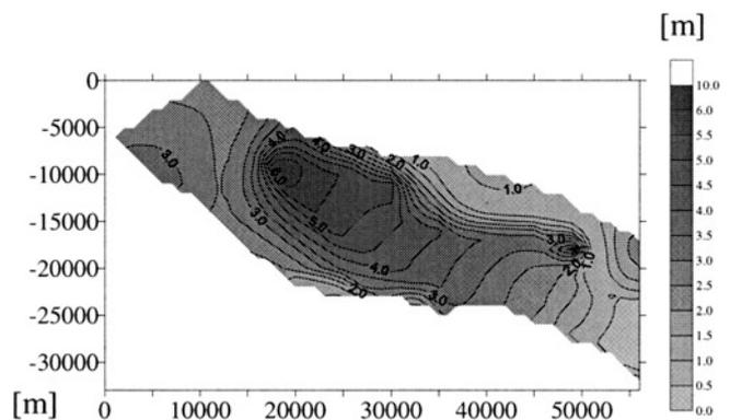
**Figure 9.** Standard deviations of heads in meters (Monte Carlo method, Palla Road Aquifer, conditioned by 10 head measurements).
