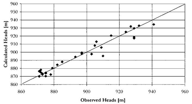
**Figure 5.** Scatterplot of observed heads versus calculated heads.
