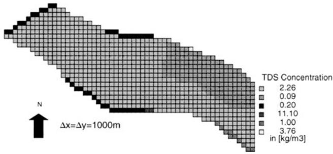
**Figure 3.** Total dissolved solids (TDS) concentration of inflows in  $\text{kg m}^{-3}$ .
