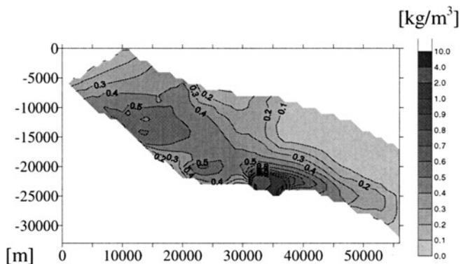
**Figure 11.** Standard deviations of concentrations in  $\text{kg m}^{-3}$  (FOSM method, Palla Road Aquifer, conditioned by 10 head measurements).
