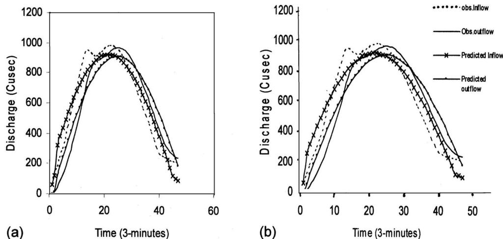
**Fig. 3.** Complete flood event prediction (Chow et al. 1988): (a) error model: predicting the error using predicted flows; (b) flow model: predicting the observed flows using predicted flow at the bounding sections obtained from initial state
