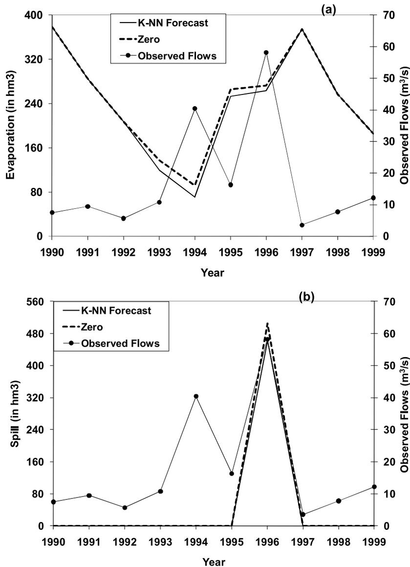
**Figure 7.** System Losses from Oros reservoir utilizing K-NN forecasts and based on Zero Inflow assumption: (a) evaporation and (b) spill. The end of the year target storage was assumed to be 260 hm<sup>3</sup> which would ensure municipal supply for an additional 18 months. The reliability of supply for each use is 90%.
