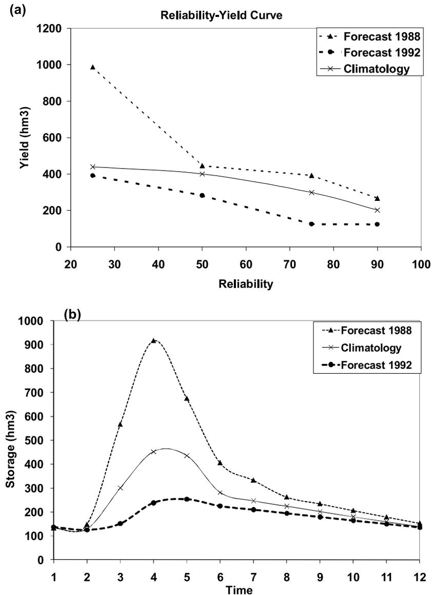
**Figure 5.** Bulk Sector Water allocation for years 1988 and 1992 for the Oros reservoir using the 12 month lead semiparametric K-NN forecast and using the climatological ensembles: (a) Reliability Yield Curve and (b) median of the simulated storages for supplying 90% reliability.
