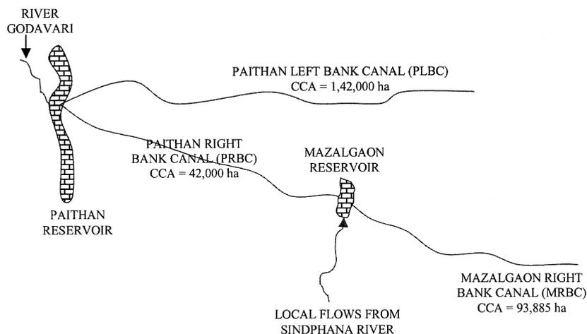
Fig. 2. Schematic diagram of Jayakwadi irrigation project.
