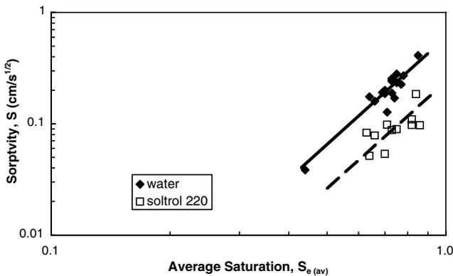
Fig. 8.  $\log_{10}(S)$  versus  $\log_{10}(S_{e(av)})$ . The solid line is the power law  $S = 0.6S_{e(av)}^{3.2}$ . The dashed line is the power law  $S = 0.24S_{e(av)}^{3.2}$ .
