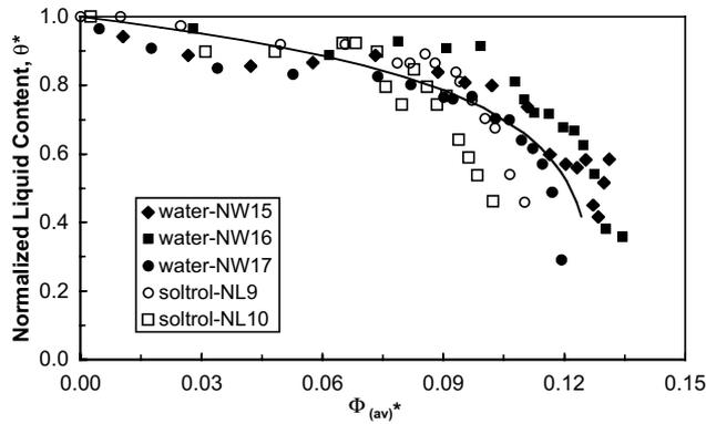
Fig. 10.  $\theta^*(x, t_{\text{end}})$  versus  $\Phi_{av}^*$ . The solid line is the approximation provided by Eq. (26) using  $m = 6$  and  $s_{av}^* = 0.105$ .
