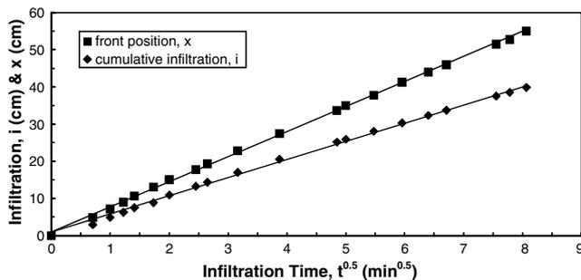
Fig. 4. Plot of  $i(t)$  versus  $t^{1/2}$  for *NW8*, an experiment conducted using water as the infiltrating fluid in a circular tube. The inlet head  $h_0 = +5$  cm. The linear relationship between  $x(t)$  and  $t^{1/2}$  is also displayed.
