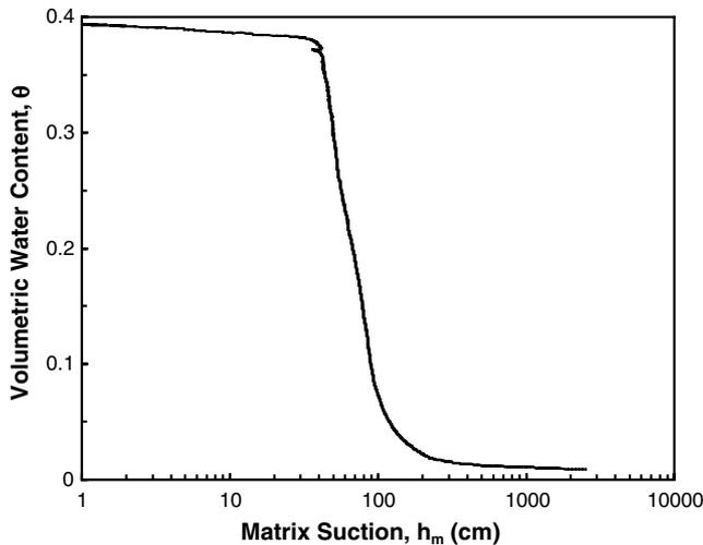
Fig. 1. Soil moisture characteristic curve of the sand during drying. The sand was packed at a porosity  $n = 0.4$  and fully saturated using deaired pure water at high pressure before drying commenced.  $\theta$  is the volumetric water content of the sand and  $h_m$  is the measured metric suction in cm of water.
