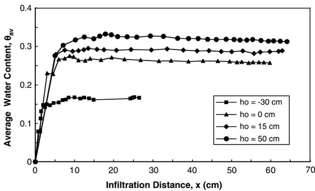
Fig. 5.  $\theta_{av}(t)$  versus  $x(t)$  for select water infiltration experiments.
