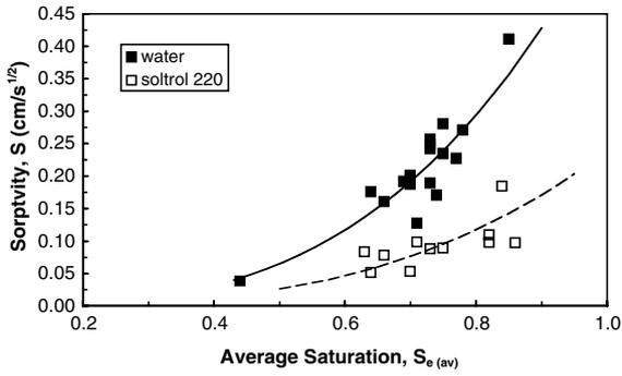
Fig. 7. Observed relationships between  $S$  and  $S_{e(av)}$ . The solid line is the power law  $S = 0.6S_{e(av)}^{3.2}$ . The dashed line is the power law  $S = 0.24S_{e(av)}^{3.2}$ .
