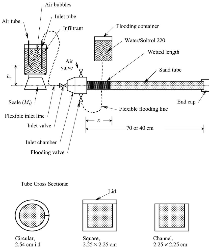
Fig. 2. Schematic diagram of experimental apparatus.
