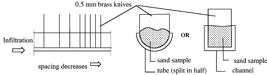
Fig. 3. Sampling for liquid content measurements at the end of an experiment.
