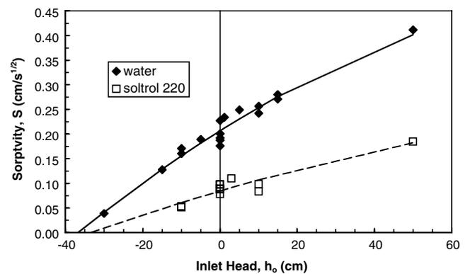
Fig. 6. Observed relationships between  $S$  and  $h_0$ . The symbols are experimental data. The lines are empirical relationships between  $S$  and  $h_0$  that assume a second order polynomial. The fitted relationship for the water (solid line) is;  $S_w = -2 \times 10^{-5}h_0^2 + 0.0049h_0 + 0.207$ ;  $R^2 = 0.97$ , while that for the Soltrol 220 (dashed line) is  $S_o = -7 \times 10^{-5}h_0^2 + 0.0023h_0 + 0.0845$ ;  $R^2 = 0.88$ .
