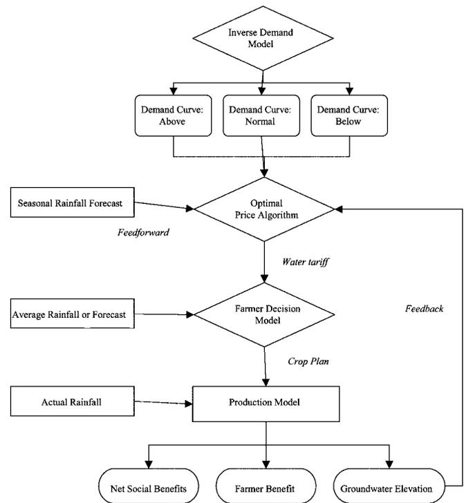
Fig. 2. Schematic of simulation model
