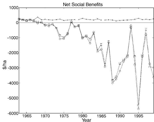
**Fig. 4.** NSB in \$/ha of three pricing models for the 37-year simulation. The trajectories shown are for the fully adaptive model (solid line with x's), the feedforward model (line with squares), and the static model (line with circles). The fully adaptive pricing model results in continuously positive NSB averaging about \$170/ha, while the feedforward and static models yield steadily decreasing NSB.
