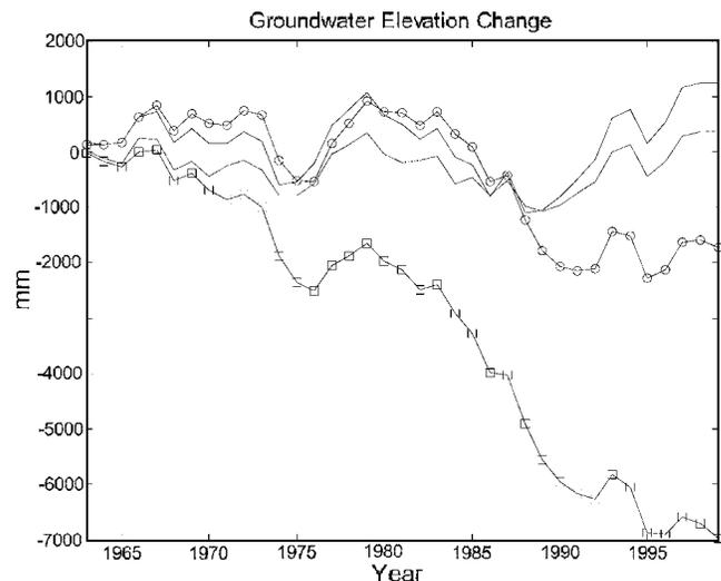
**Fig. 7.** Effect of recharge on groundwater elevation. Groundwater elevation over the 37-year simulation for a recharge rate of 100% of rainfall (black line=fully adaptive model; line with circles=static model) and a recharge rate of 70% of rainfall (blue line=fully adaptive model; line with squares=static model). Higher recharge rates decrease the gap between groundwater elevations produced by the adaptive pricing and static pricing models to some extent.
